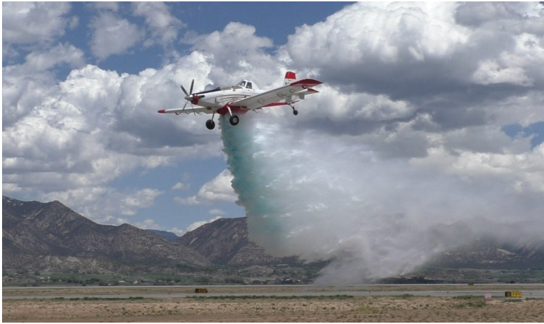
A Single Engine Air Tanker (SEAT) drops water with polymer mixed in during testing. Photo courtesy of the Center of Excellence.
